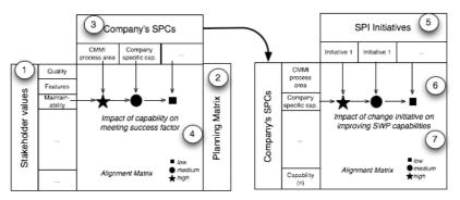
Figure 1: Overview of the method for aligning stakeholder values, software process capabilities, and SPI initiatives.
